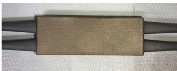
Fig. 3. Enhanced mockup by using 3D metal printing with Al-bronze powder
