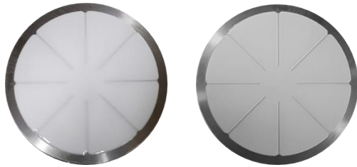
Fig. 8. Aqueous suspension (PMMA powder dispersed in the DI water) on the powder mold(left) and dried powder film(right): thresholds are prepared to minimize non-uniform distribution.
