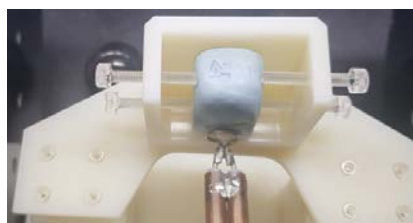
Fig. 2. The teeth phantom was position at surface coil of resonator. The phantom was inserted into custom-made immobilization frame made of non-magnetic material polycarbonate which is non-magnetic material.
