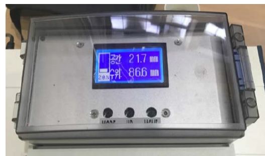
Figure 2. Water Level Displayer
