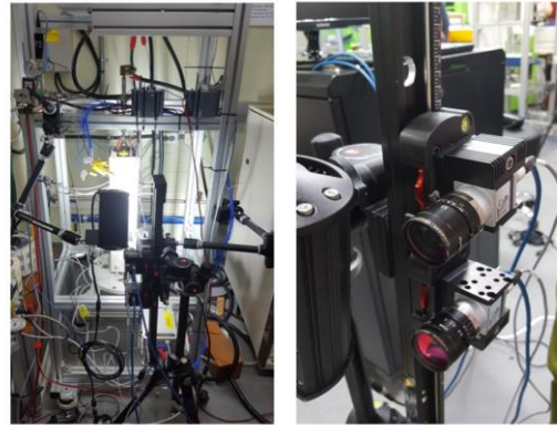
Fig. 3. Photograph of ‘FISRBIT’ facility equipped with components for DIC measurement.
