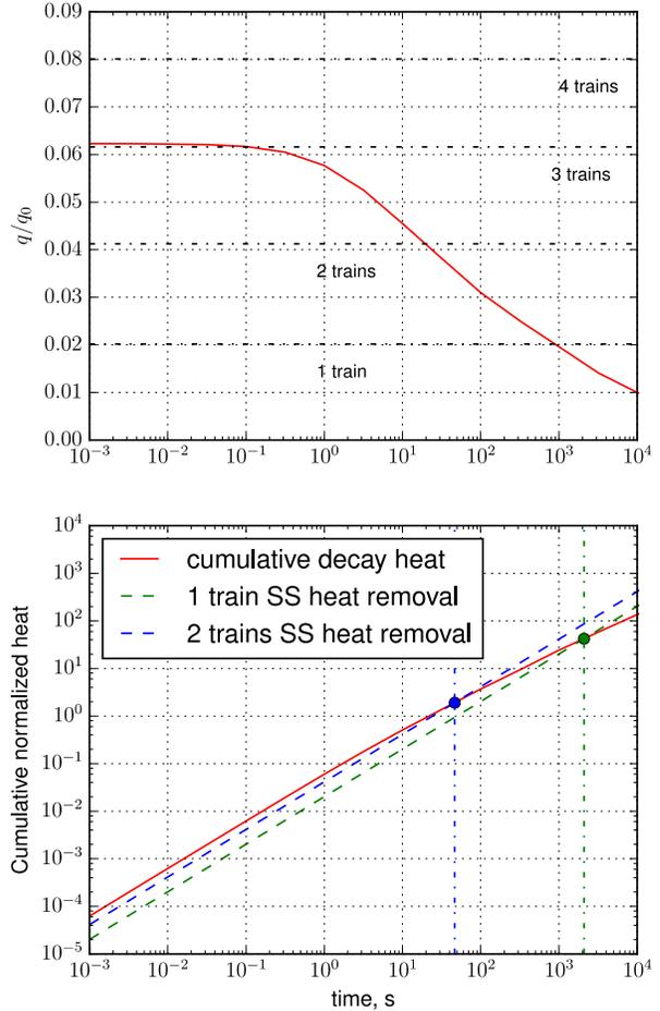
Fig. 4. Observed steady-state heat removal capacities compared to a typical normalized decay heat curve.
