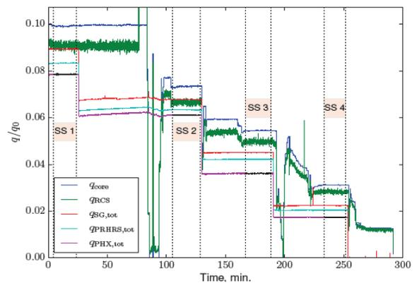
Fig. 3. Selection of the Measured Variables Related to the PRHRS System Performance
