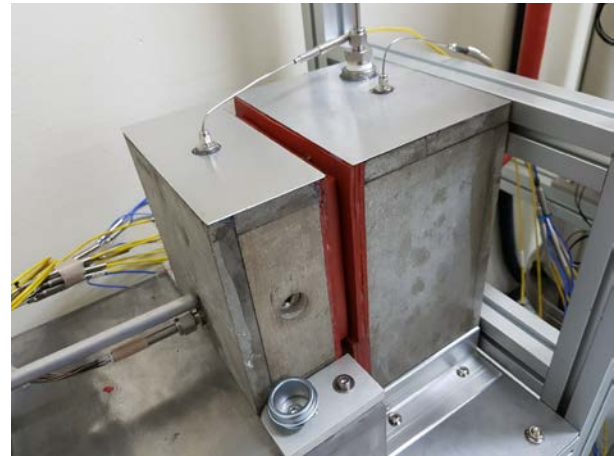
Fig. 6. Close-up photo of heat transfer module with the PCM chamber (left) & steam chamber (right)
