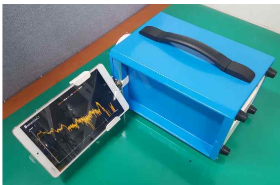
Fig. 4. 3 rd Quad-CZT Array (Wireless Network System)
