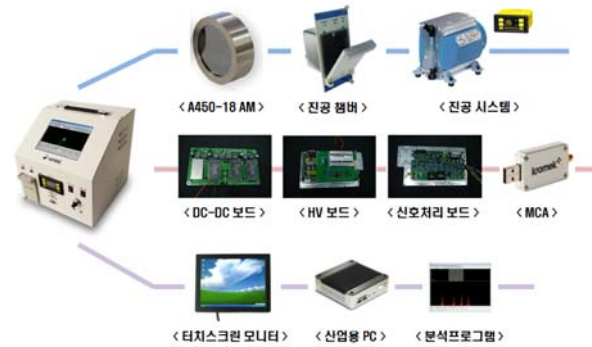
Fig.5. A portable alpha-particle spectrometer developed by KINAC
