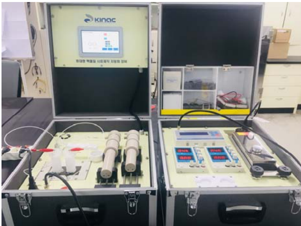
Fig.4. Developing automated nuclear material sampler
