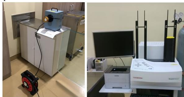
Fig. 2 The air-sampler (left) used to collect the air near the entrance of the radiation controlled area (A1) and the low alpha-beta counter (right) used to measure the radioactivity of the filter installed in the air-sampler.
