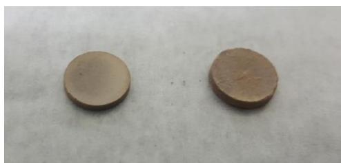
Fig. 3. \text{CeO}_2 - \text{Ce}_3\text{Si}_2 composite pellets fabricated by microwave sintering at 1500 °C for 1 h.
