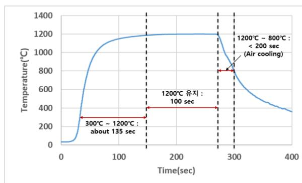
Fig. 1. The temperature profile of the specimen during the oxidation testing
