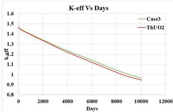
Fig. 4. Behavior of k-eff of ThUC and ThUO2 loaded core with operation time.
