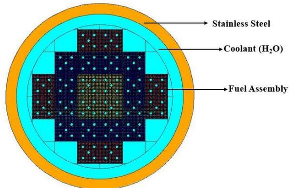
Fig. 1. Core configuration of thorium carbide small reactor
