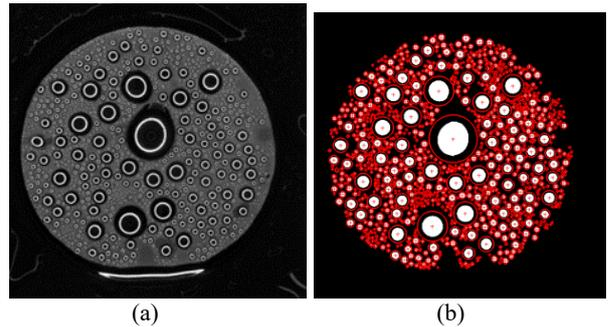
Fig. 5. (a) Visualization of condensing surface, (b) Image processed result
