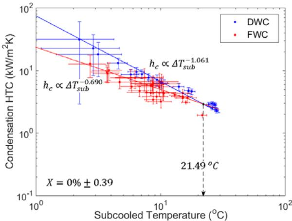
Fig. 4. Comparison of condensation HTC between DWC and FWC phase at pure steam condition
