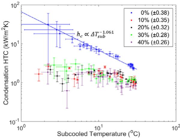
Fig. 3. Subcooled temperature versus condensation HTC
