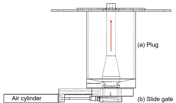
Figure 2. Nozzle opening system;
