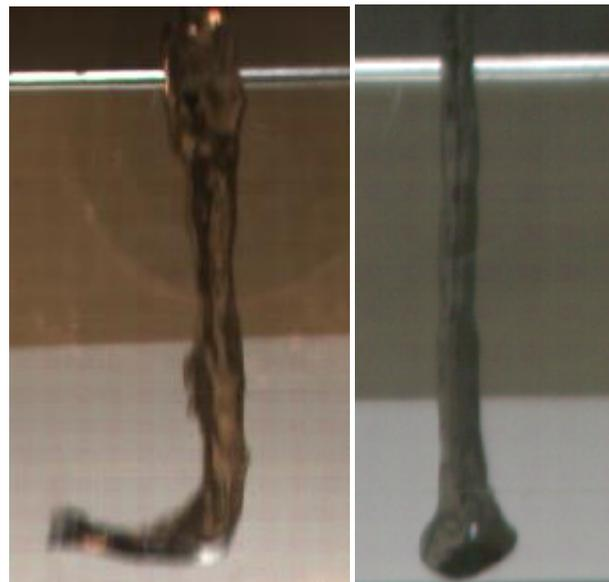
Figure 3. Melt jet shape before entering the water surface with same nozzle diameter; (left) MATE09 (without slide gate), (right) MATE14 (with slide gate)
