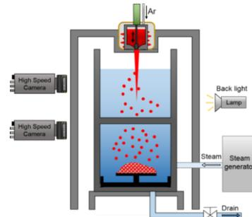
Figure 1. Schematic figure of the MATE facility
