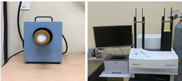
Fig. 1 The air-sampler (left) used to collect the air near the shielding door in the preparing room and the low background alpha-beta counter (right) used to measure the activities for the alpha and beta on the filter, which installed in the air-sampler.
