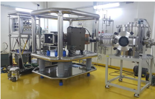
Fig. 3. Alkali metal ion implanter under construction.
