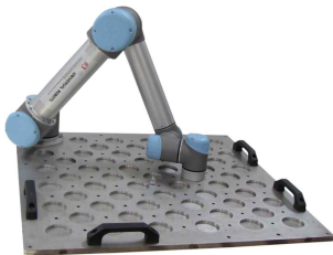
Fig. 3. Calibration plate with holes to align the end effector
