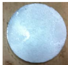
Fig.2. Salt-Ingots prepared at 500°C.
