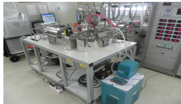
Fig. 4. Experimental apparatus for the in-bed calorimetry
