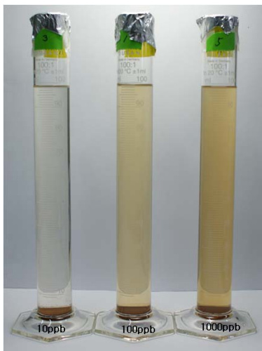
Fig. 1. Settling test results as a function of PAA concentration (50 ppm magnetite, 7 days suspension)
