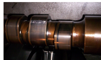
Fig. 3 Damaged fuel cam lobe
