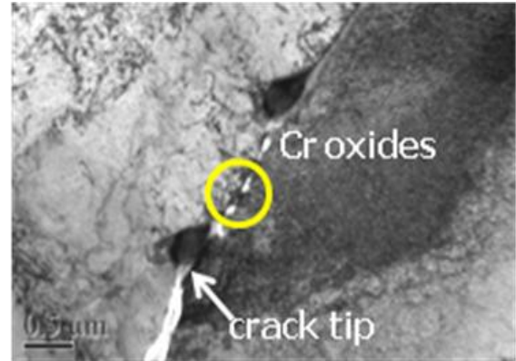
Fig. 5 TEM bright field image taken on the leading grain boundary ahead of the crack tip.
