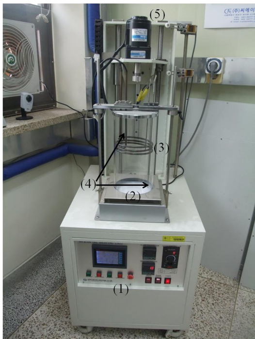
Fig. 3. Schematic figure of the oil-bath furnace. (1) controller; (2) heating plate; (3) heating coil; (4) thermal couples; (5) rotating and pulling motors.
