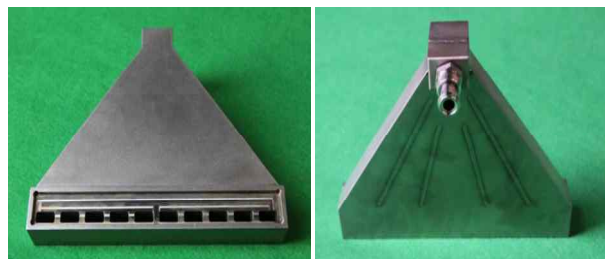
Fig. 3. Photo of the fabricated manifold
