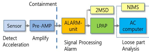
Fig. 1. The schematic diagram of the major components of LPMS of OPR-1000
