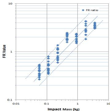
Fig. 3. FR diagram for Channel #9 of LPMS of Shin-wolsung NPP unit 1.
