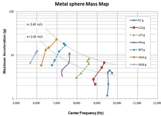
Fig. 2. Metal Sphere Mass Map for Channel #9 of LPMS of Shin-wolsung NPP unit 1.
