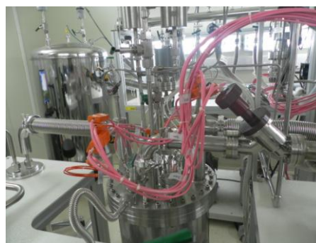
Fig. 3. Apparatus of a hydrogen storage bed.
