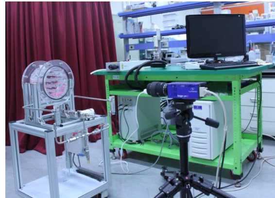
Fig. 1. PIV system with a scaled-down Calandria vessel
