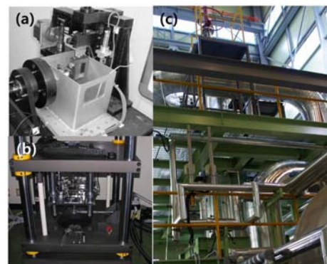
Fig. 1. Experimental facilities of nuclear fuel fretting; (a) part unit (b) 1x1 cell unit; (c) F/A unit.
