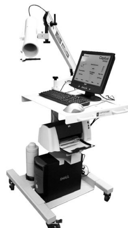
Fig. 1 Thyroid uptake and well count system (CAPTUS 3000 CAPINTEC. Inc. U.S.A)
