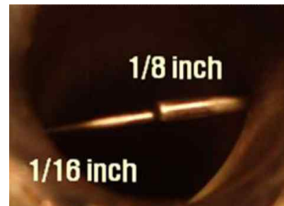
Figure 2 Two Thermocouples in the Pipe [3]
