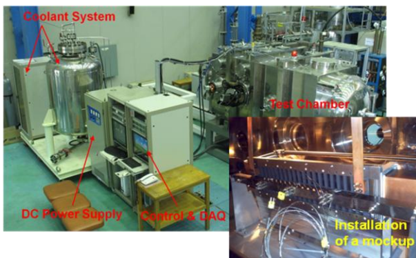
Fig. 5. Picture of KoHLT-2 and installation of a mock-up
