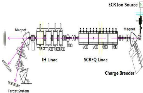
Fig. 2. Schematic of the Stable heavy-ion accelerator applied to ECR ion source and multiple purpose target system
