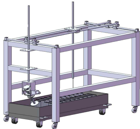
Fig.2 SG Mockup for Ultrasonic Cleaning
