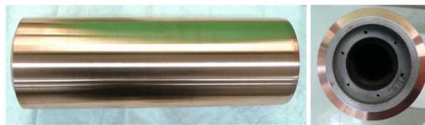
Fig. 1. Copper-cast iron disposal canister at 1/10 scale fabricated by cold spray coating.
