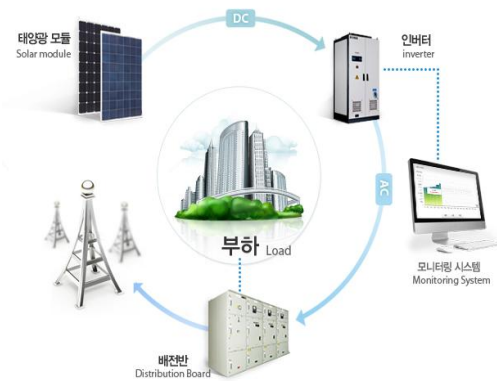
Fig 2. Monitoring System of Solar Power System
