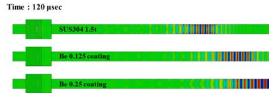
Fig. 6. Simulation results of the propagation and radiation of in the ultrasonic waveguide coated sensor at 120 μsec.
