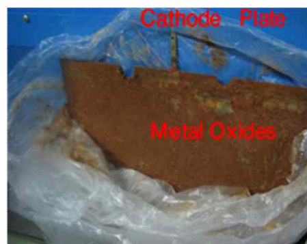
Fig. 1. Cathod plate covered with metal oxides.
