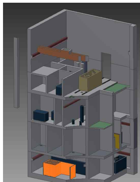
Fig.5 Internal View of Fuel Building
