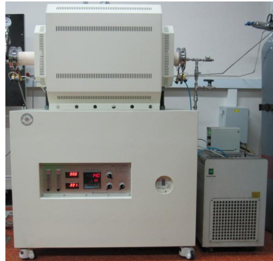
Figure 1. Apparatus (tube furnace) for high temperature oxidation of Zr alloys in air
