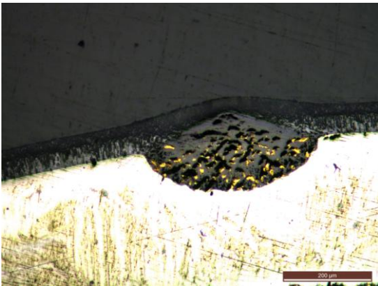
Figure 4. The microstructure of a Zirlo cladding oxidized in air at 1200C for 5 minutes.
