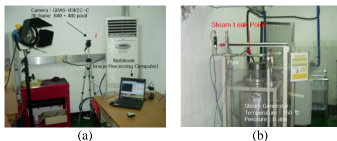
Fig. 1 Experimental setup for detecting steam leakage Camera and image processing computer, Steam generator
