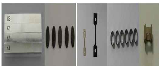
Fig. 3. Specimens(L: STS 304L & carbon/R: Zry)
