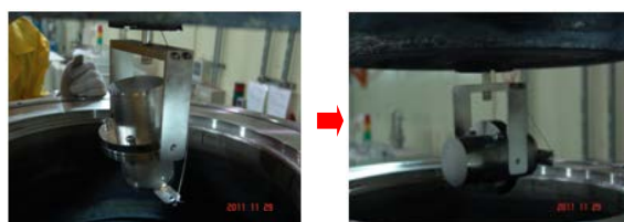
Fig. 2. Photograph of an integrated sieve-crucible assembly in the top flange of the vacuum distillation tower.
