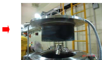
Fig.3. Rotation of the integrated sieve-crucible assembly in the salt distillation tower.
