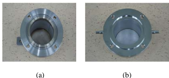
Fig. 1. Photographs of (a) a sieve for the solid-liquid separation and (b) a crucible for the integrated sieve-crucible assembly.
