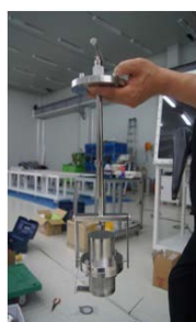
Fig. 2. Photograph of an integrated sieve-crucible assembly in the top flange of the vacuum distillation tower.
