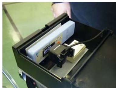
Fig. 2. Radiation measuring unit of the Quince robot
