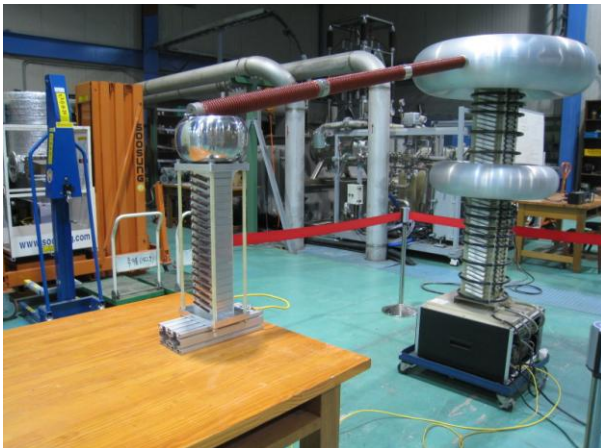
Fig. 5. High voltage test of a multi-layer DC break
