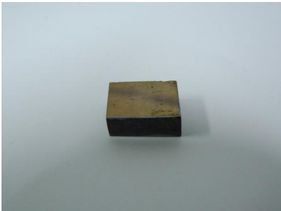
Fig. 1. CdZnTe detector with gold chloride solution electrode (10mm(W) x 12mm(L) x 5mm (T))
