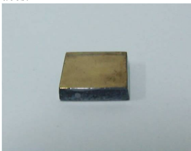
Fig. 1. The fabricated CdZnTe nuclear radiation detector by using the 6-zone LPB at KAERI.
