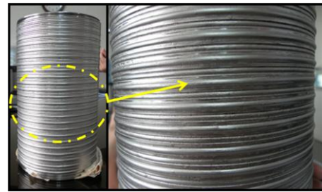
Fig. 2. Primary vessel brazed two-cable-heater.
