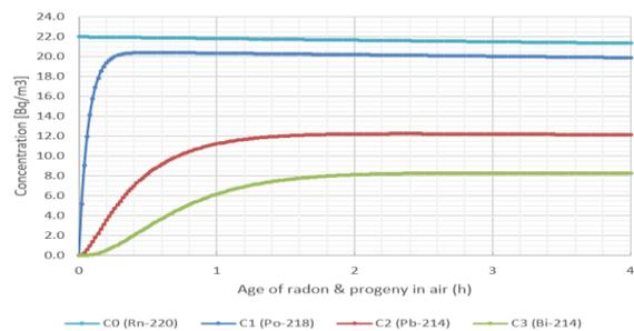
Fig. 2 Concentration change trend of radon and radon progeny when the initial concentration of radon progeny is zero.
