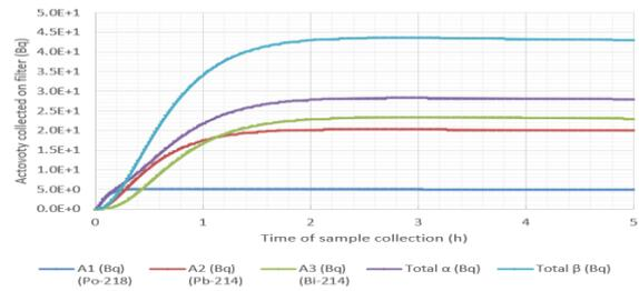
Fig. 4 Activity of radon progeny collected on filter with the time of sample collection when the deposition rate for all radon progeny is  $1 \text{ h}^{-1}$
