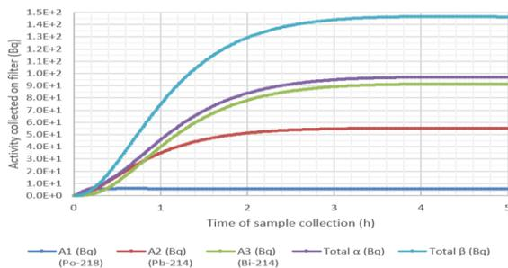
Fig. 3 Collection and ingrowth of radon progeny on filter.
