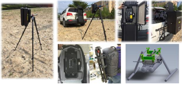
Fig. 2. Application of a multipurpose ERS system to the mobile and ground based gamma-ray spectrometry
